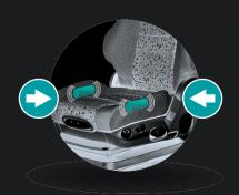
To minimise this risk, the seat will immediately start vibrating to alert you. The motors are concealed within the seat cushion warning you to take immediate action without causing unnecessary distress to your passengers.
